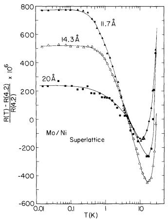
Fig. 2 Temperature dependence of normalized resistance for non-
