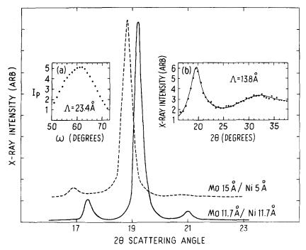
Fig. 4 00% X-ray diffraction profiles for two samples showing coherent satellites. Inset (a): Rocking curve
